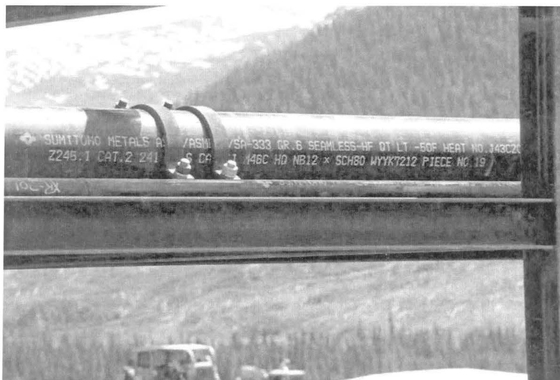
Multiple marking of ASME SA-333 Grade 6, and CSA Z245.1 Grade 241 Cat. 2.
