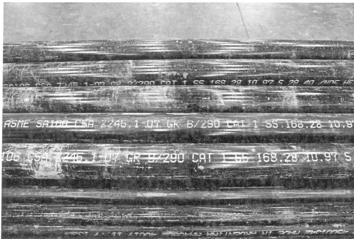
Multiple marking of ASME SA-106 Grade B and CSA Z245.1 Grade 290 Cat. 1.
